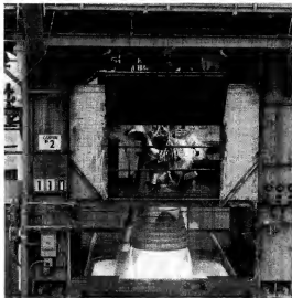
At left is shown a 1963 test firing of an H-1 engine on a Rocketdyne test stand. At right are H-1 engines in Rocketdyne's assembly line at Canoga Park, California.
